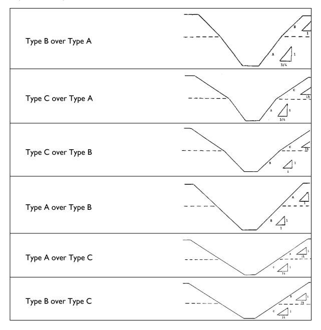
All other sloped excavations must be in accordance with the other options described in Section 11 – Sloping and Benching Systems.
