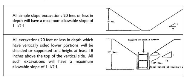
All other sloped excavations must be in accordance with the other options described in Section 11 – Sloping and Benching Systems.
