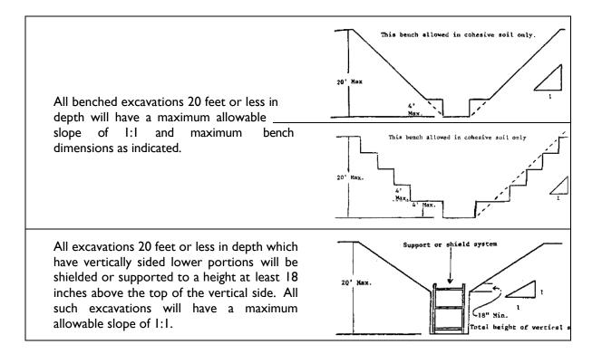
All other sloped excavations must be in accordance with the other options permitted in Section 11 – Sloping and Benching Systems.
