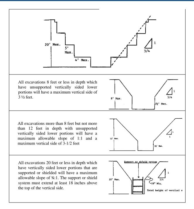
All other simple slope, compound slope, and vertically sided lower portion excavations will be in accordance with the other options described in Section 11 -Sloping and Benching Systems.
